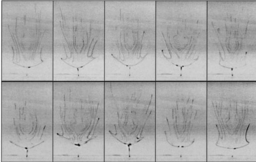
FIGURE 12. Dye sheet released from the centre of the bottom stationary endwall for  $Re = 3600$ . Images are equally spaced over a time  $\tau_3$  of the  $\tau_3$  quasi-periodic flow, using one frame per image. The images depict a subset of the meridional plane  $r < 0.4R$  and  $0 \leq z < 0.5H$ , illuminated by a laser sheet.
