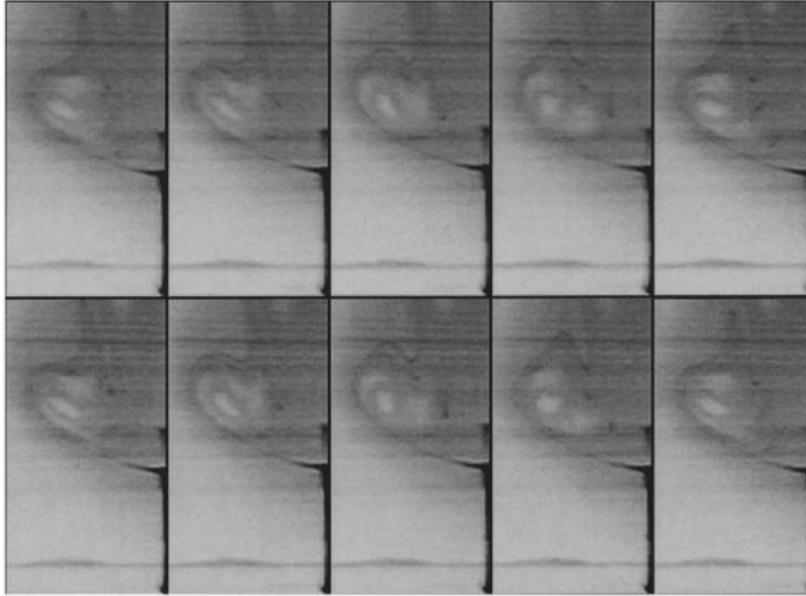
FIGURE 4. Closeup view of the dye sheet released from the centre of the bottom stationary endwall for  $Re \approx 2700$  showing a period-one elliptic region surrounded by period-two islands; frames cover two complete  $\tau_1$  periods.
