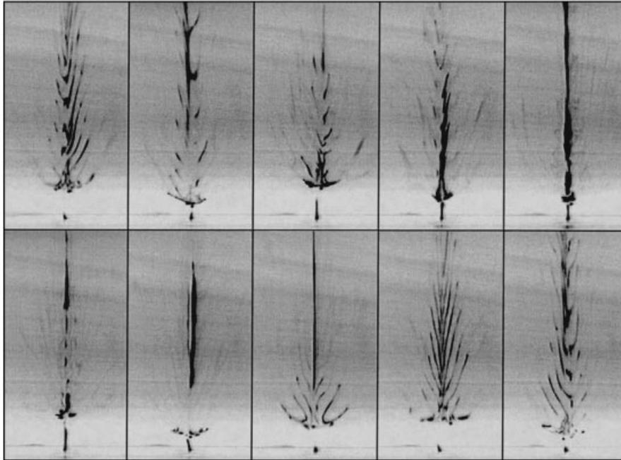
FIGURE 13. Dye sheet released from the centre of the bottom stationary endwall for  $Re \approx 4400$  from time  $\Omega t = 0$  to 1388. Images are equally spaced and constructed with 1 frame per image.
