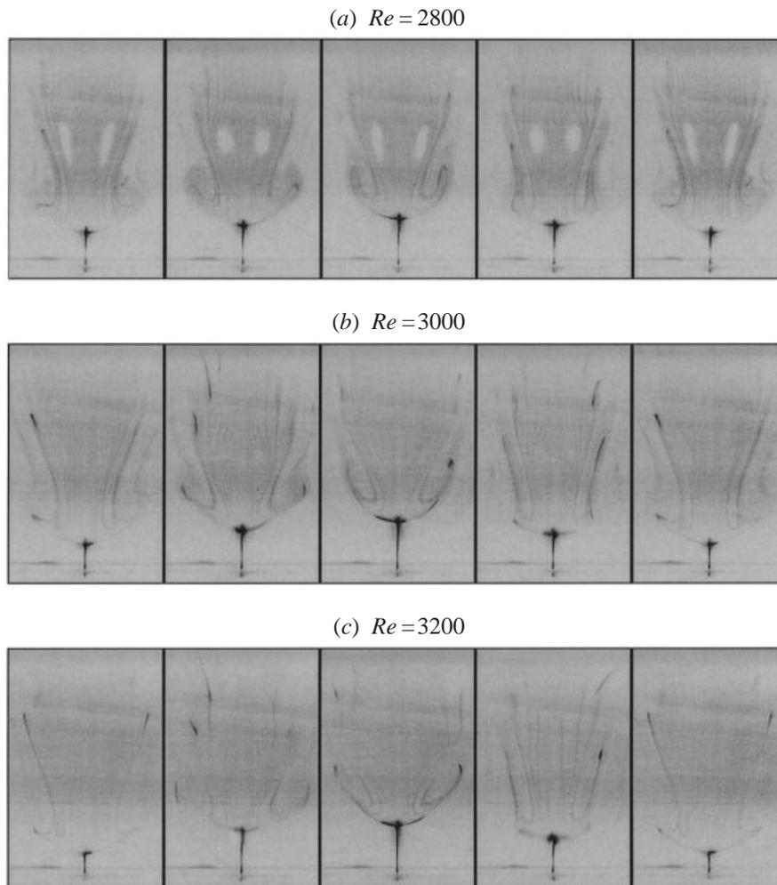
FIGURE 3. Dye sheet released from the centre of the bottom stationary endwall for (a)  $Re = 2800$ , (b)  $Re = 3000$ , and (c)  $Re = 3200$ . Images are equally spaced over a period of  $\tau_1$  and are composed of 30 frames each at the same phase. They depict a subset of the meridional plane  $r < 0.4R$  and  $0 \leq z < 0.5H$ , illuminated by a laser sheet.
